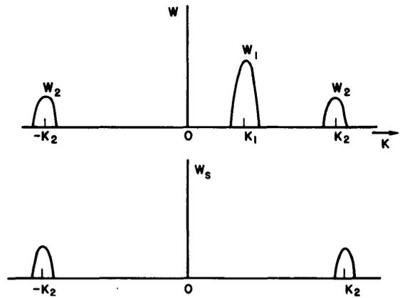
FIG. 3. Two-stream ( $W_1$ ) and parametrically created daughter waves ( $W_2, W_s$ ).
