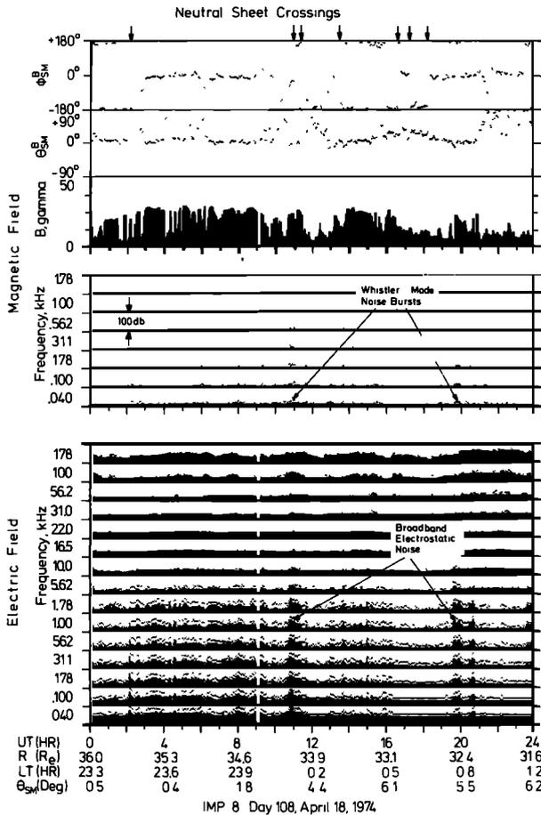
Fig. 5. Magnetic field and plasma wave measurements made by the Imp 8 spacecraft for day 108 during a transit of the neutral sheet [Gurnett *et al.*, 1976]. Note the intense electrostatic and magnetic noise bursts which occurred throughout the day.
