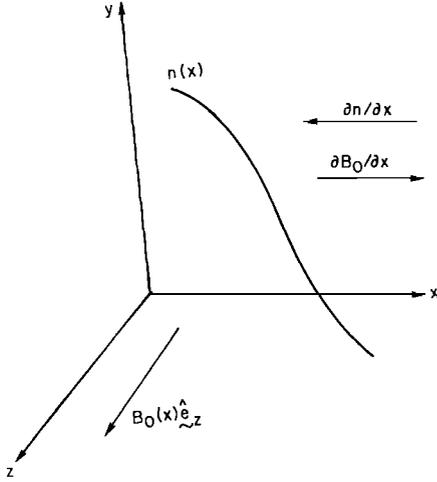
Fig. 1. Slab geometry and background plasma configuration.
