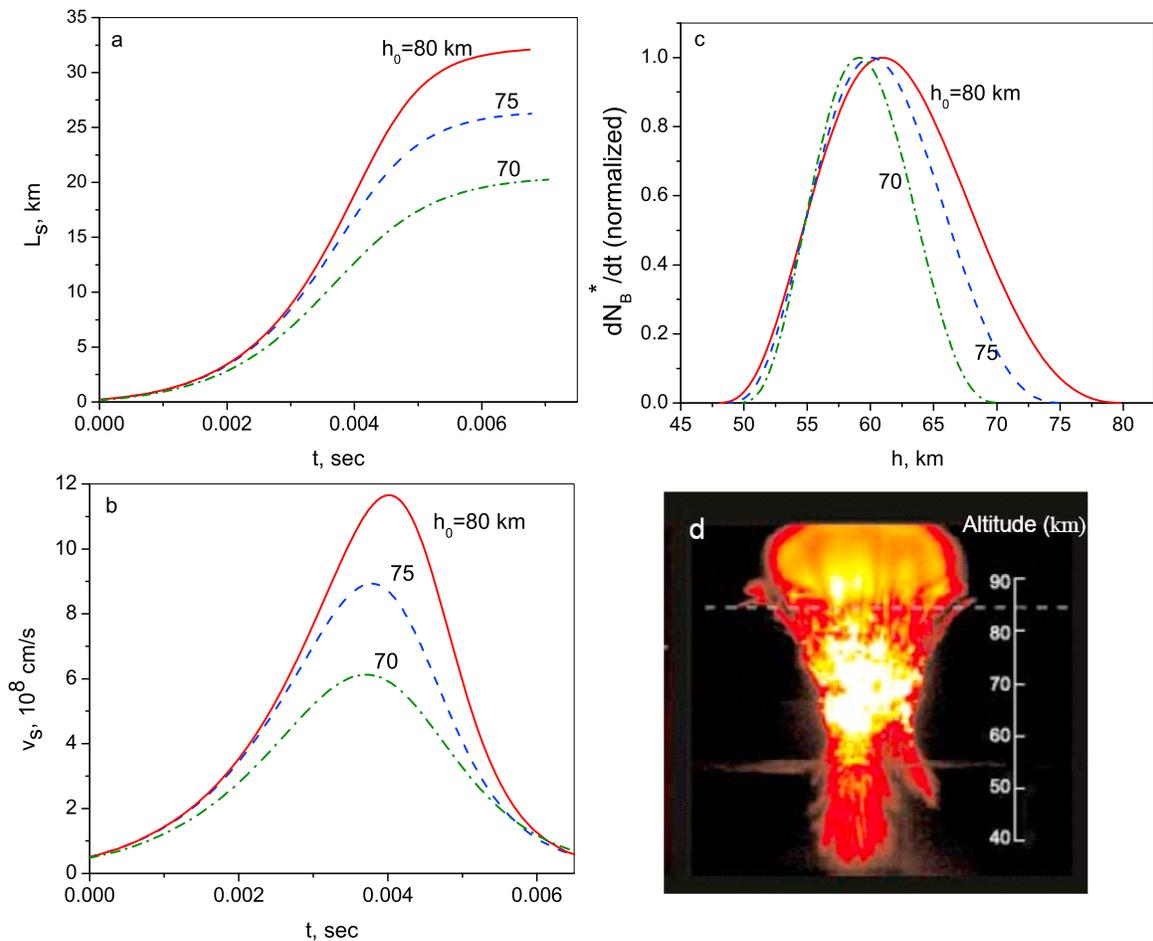
**Figure 6.** (a) The length of the streamers versus the propagation time. Here the streamers were launched from the different altitudes. (b) Same for the streamer velocity. (c) The excitation rate of  $N_2(1P)$  emission normalized by its peak value, generated by the streamers launched from the different altitudes. (d) Photo of red sprites (adapted from *Stenbaek-Nielsen and McHarg* [2008] with permission).
