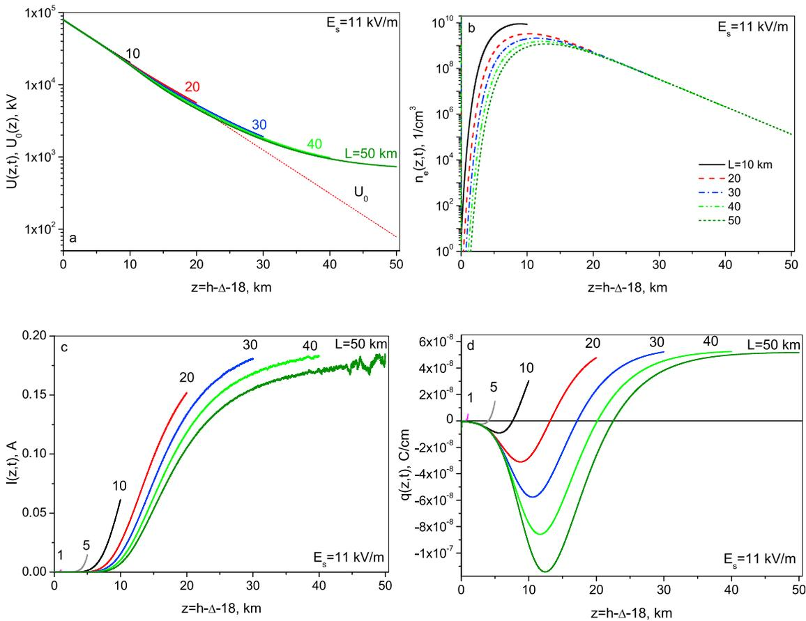
**Figure 11.** Results of numerical computations of a long streamer growing in the exponential atmosphere and in the exponentially changing external field. Thus, the similarity law holds. (a) The potential distribution along the streamer channel computed at different times when the streamer’s length is 5, 10, 20, 30, 40 or 50 km. (b) Respective distribution of the electron density. (c) Current distribution. (d) Charge per unit channel.
