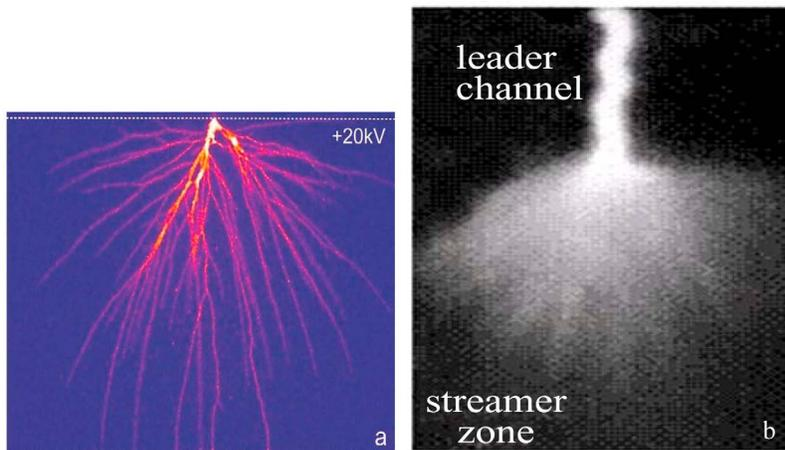
**Figure 1.** (a) A photograph of a positive streamer in a 40 mm gap in air at 1 bar (adapted from *Briels et al.* [2008] with permission). (b) A photograph of a positive laboratory leader (adapted from *Raizer et al.* [2007] with permission from Elsevier).
