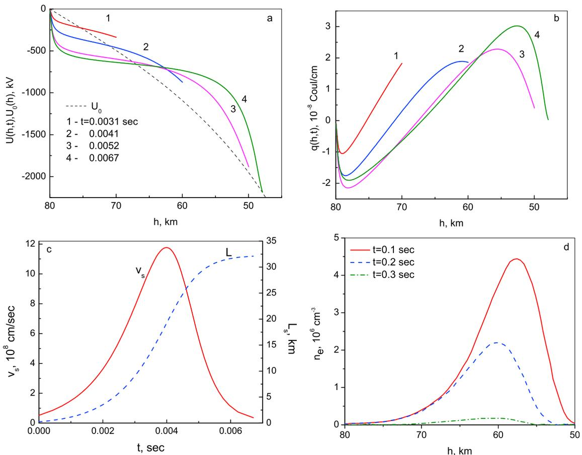
**Figure 5.** (a) Distribution of the streamer tip potential along the streamer channel computed for a few consecutive times. The dashed line shows the external potential. (b) Distribution of the linear streamer charge along the streamer channel. (c) The streamer velocity is shown by the solid line, and its length is shown by the dashed line. (d) Electron density in the streamer channel computed for the different times.
