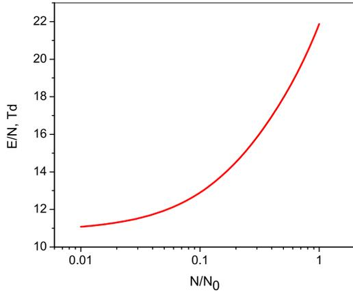
**Figure 10.** Values  $E_s/N$  required for the streamer growth versus the air density.
