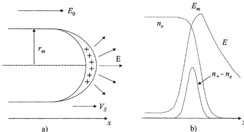
**Figure 2.** (a) Schematic diagram of a streamer tip and the leading part of the streamer channel. (b) The qualitative distribution of the electron density  $n_e$ , field  $E$ , and the difference between the densities of positive ions and electrons which defines the space charge density, along the streamer axis.
