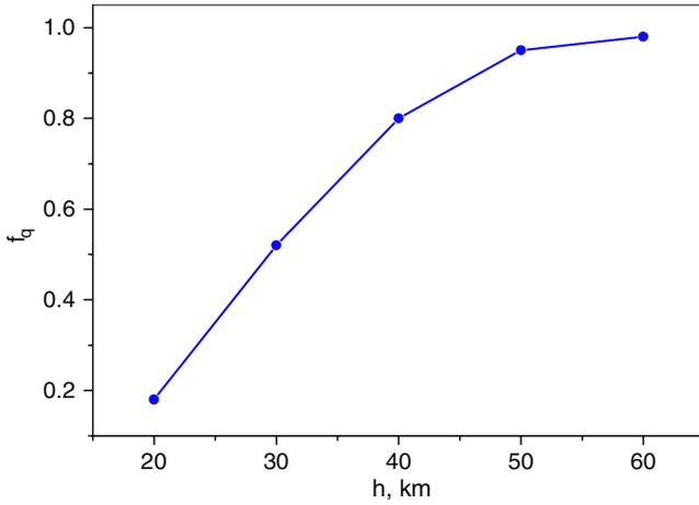
**Figure 4.**  $N_2(C)$  quenching coefficient  $f_q$  in the atmosphere versus altitude.
