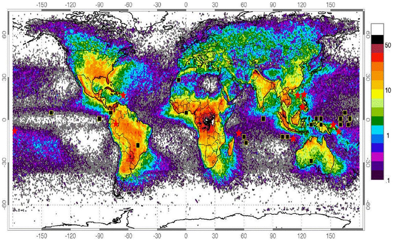
**Figure 1.** Global lightning map with superimposed locations of GBJ events (stars) and UV flashes (squares) detected by the ‘Tatiana’ microsatellite. The colour scale shows the rate of lightning appearance given in flashes  $\text{km}^{-2} \text{year}^{-1}$ . (Colour online.)
