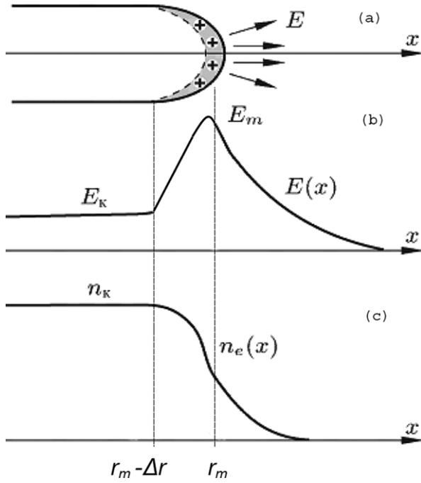
**Figure 2.** Schematic diagram of a streamer tip as well as the qualitative distribution of the electron density and electric field along the streamer axis.
