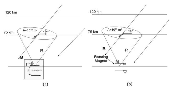
**Figure 7.** Schematic illustration of SAW injected into the ionosphere using (a) Horizontal Electric Dipole (HED) and (b) Horizontal Magnetic Dipole (HMD) antennas.
