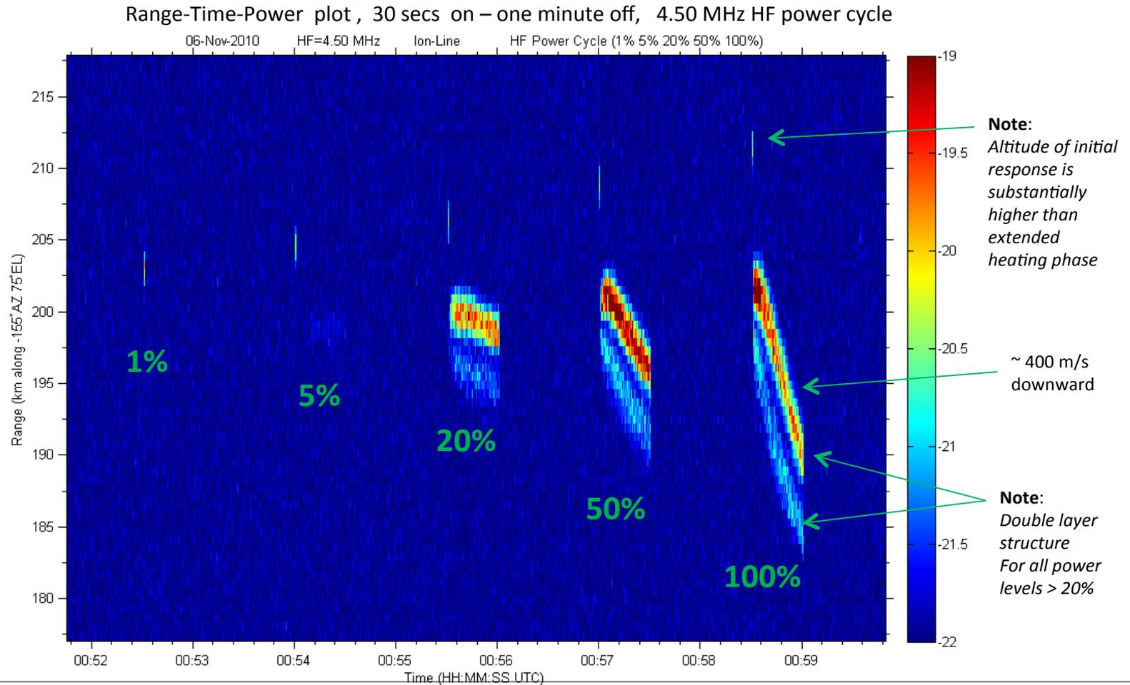
1. At least 20% of HAARP full power is required to attain substantial large-scale modification of ionospheric structure.
