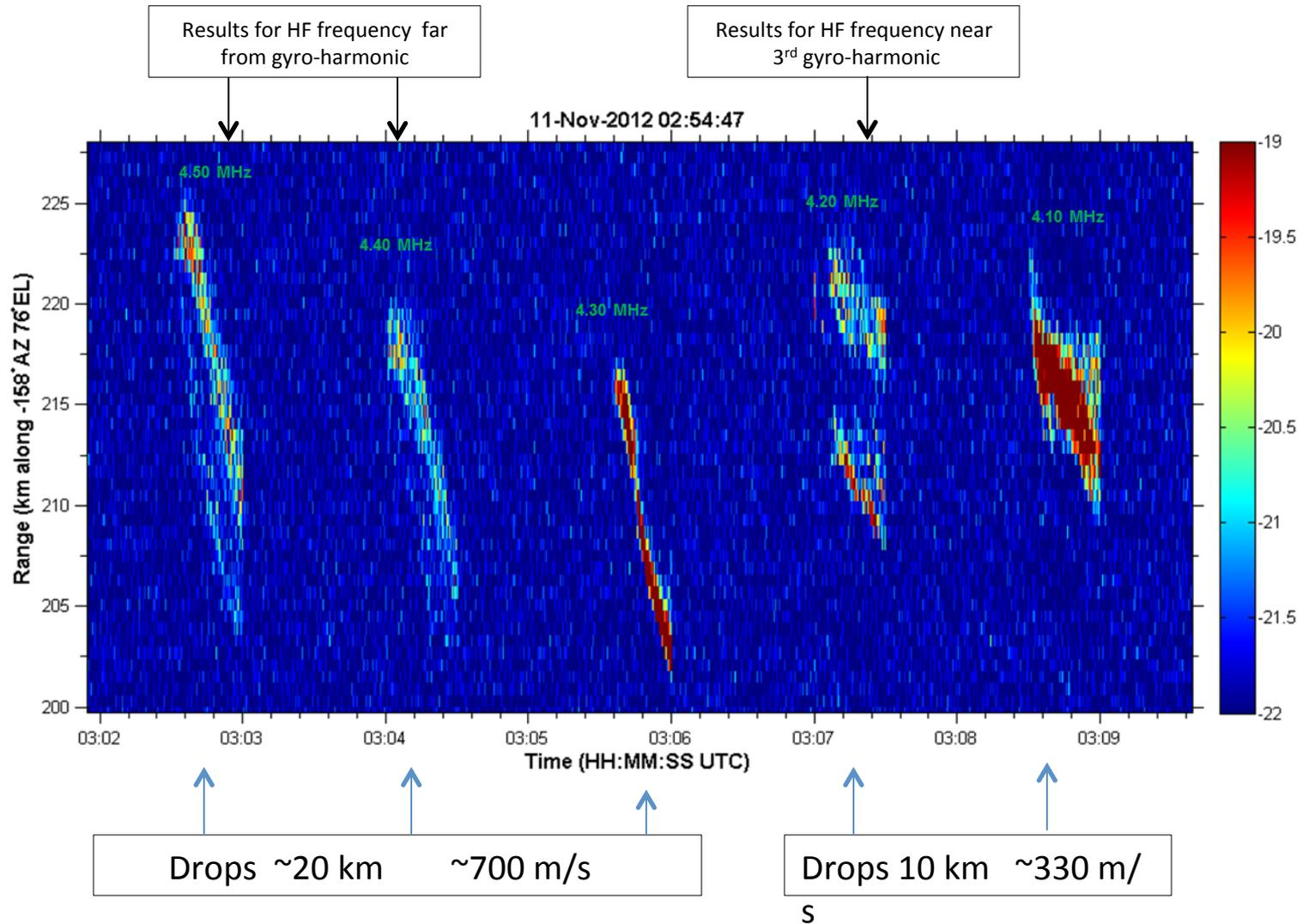
Enhanced Ion-Line Doppler Spectra for 4.20MHz
