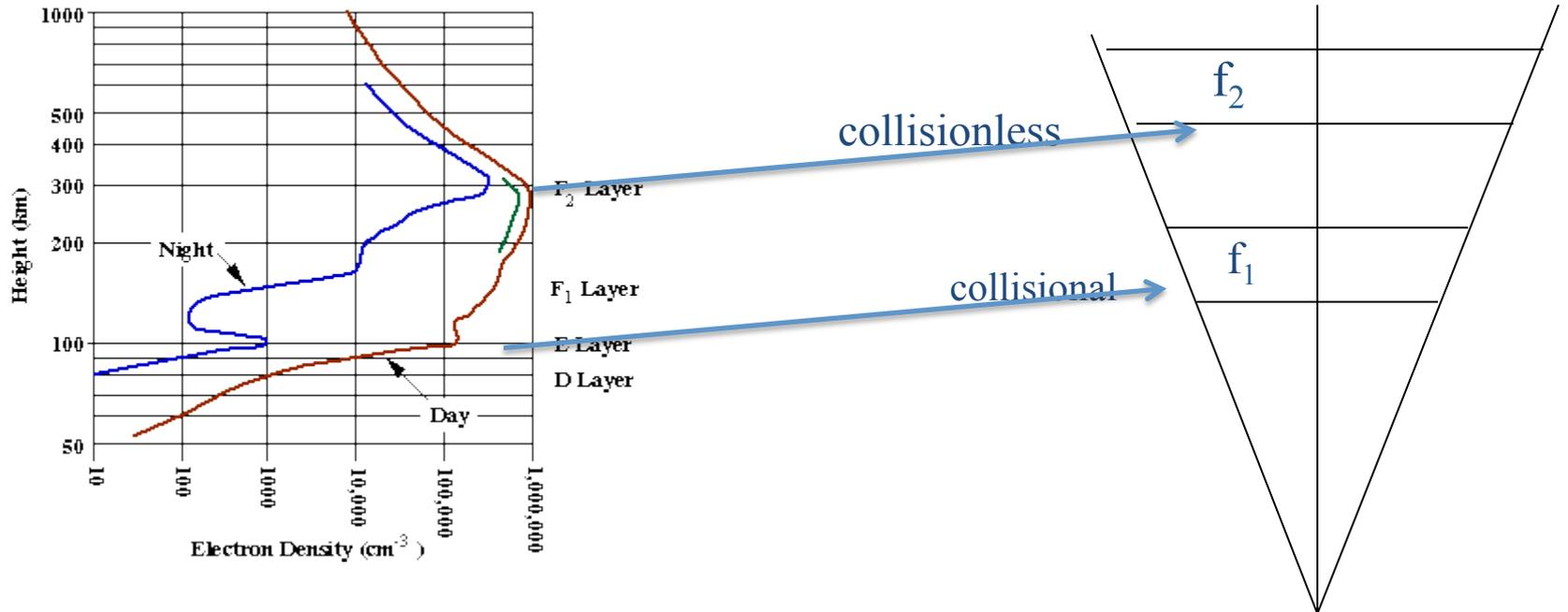
**High power RF transmitters between 2.5-10 MHz that deposit energy into the electrons at altitudes 70-100 km (D/E region) or 200-300 km (F-region) in a controlled fashion.**
