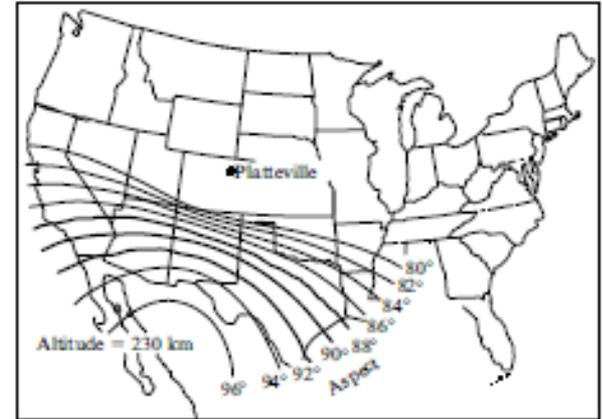
FAS Concept- Aspect scattering. RF transmitted from Tx along the 90° line are orthogonal to FAI and will be observed everywhere at the 90° line. Tx located in the 92° line observed at 88° and vice versa
