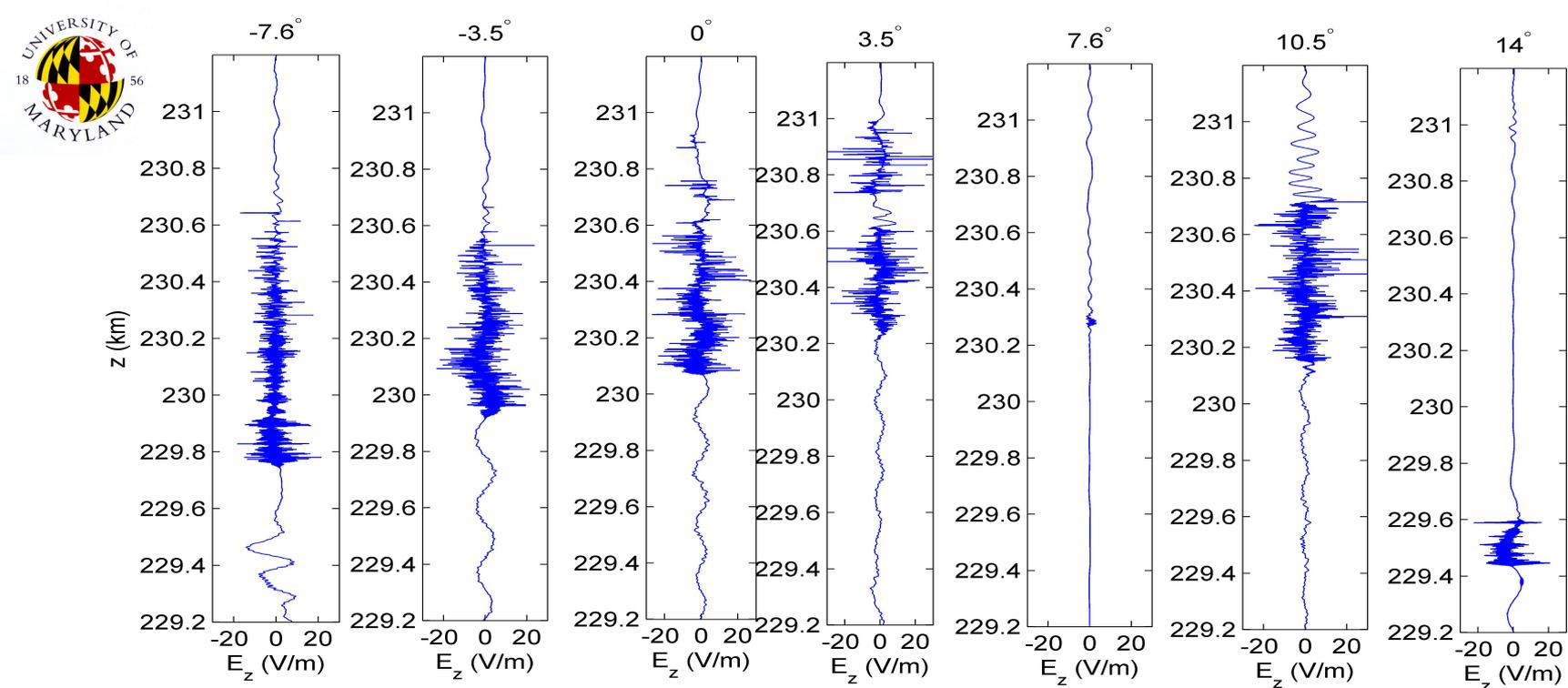
O-mode, 1V/m amplitude, electron temperature 0.4 eV, and different angles of incidence, B field *at*  $14^\circ$  to the vertical line (same parameters as JGR 2012).
