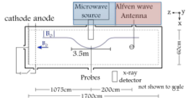
Figure 2. Linear Plasma Device (L-PPD) at UCLA. Photo by
