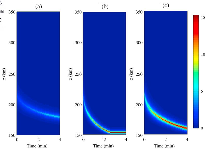
**Figure 13.** Green line emission as derived from simulation for different input wave amplitude and initial electron thermal energy: (a)  $E_0 = 1$  V/m,  $T_e = 0.4$  eV, (b)  $E_0 = 1.5$  V/m,  $T_e = 0.4$  eV, and (c)  $E_0 = 1$  V/m,  $T_e = 0.6$  eV.
