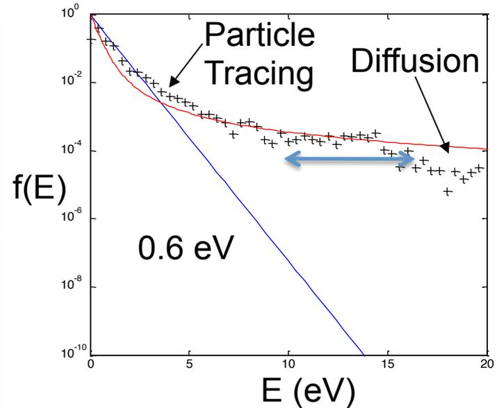
Enhancement due supra-thermal tails. Similar to Arecibo enhancement by photoelectrons but much stronger. The ionizing wave includes large  $T_e/T_i$  plasma and hot electron tails. Enhancement stops at low altitude when collisional damping dominates over Landau.
