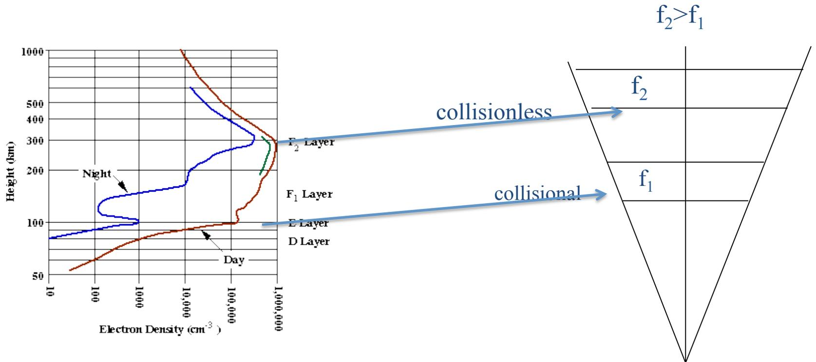
High power RF transmitters between 2.5-10 MHz that deposit energy into the electrons at altitudes 70-100 km (D/E region) or 200-300 km (F-region) in a controlled fashion.
