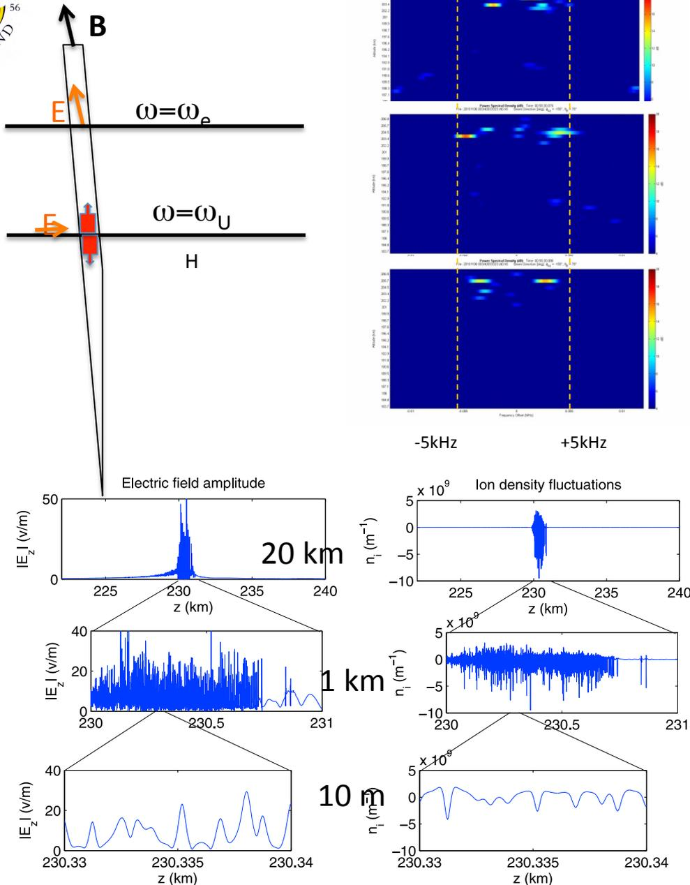
**Figure 2.** The amplitude of  $E_z$  and slowly varying ion density fluctuations  $n_i$  at various altitudes, for  $E_0 = 1.5 \text{ V/m}$ .
