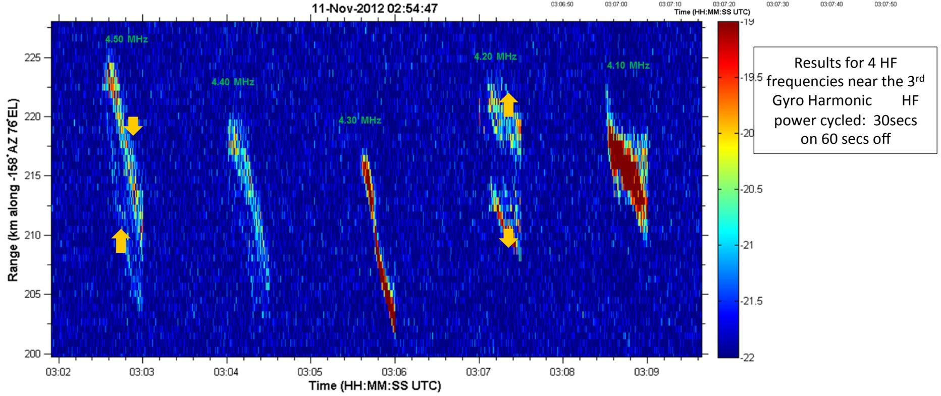
Results for 4 HF frequencies near the 3<sup>rd</sup> Gyro Harmonic HF power cycled: 30secs on 60 secs off
