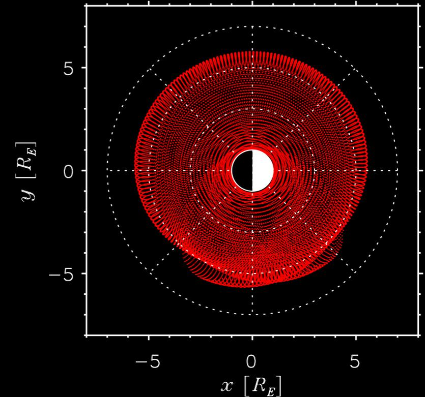
Differing apogees allow for simultaneous measurements to be taken over the full range of observatory separation distances several times over the course of the mission. Design allows one observatory to lap the other every  $\sim 75$  days.
