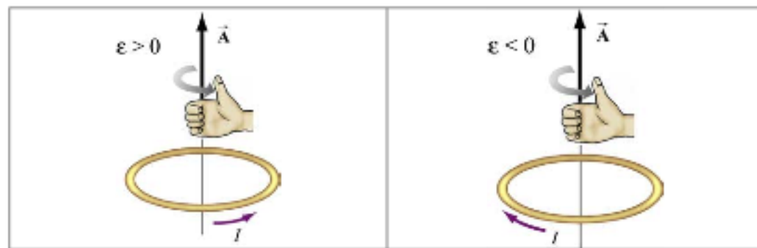
Figure 10.1.6 Determination of the direction of induced current by the right-hand rule
