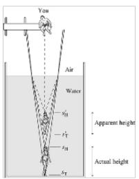
Paraxial rays from the head and the toes of the diver refract into the air and then enter into your eyes. When these refracted rays are extended into the water, the head and the toes appear elevated toward you.
